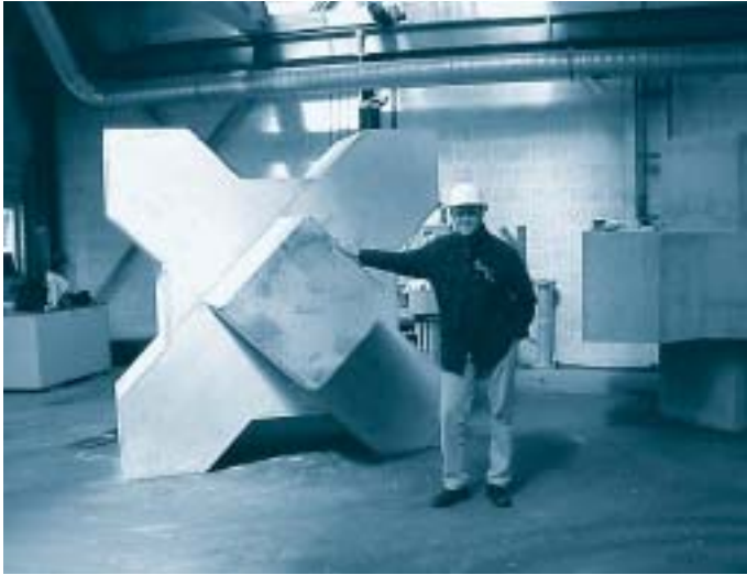
Figure 1. The 4 m 3 Xbloc ® with one of the engineers.
