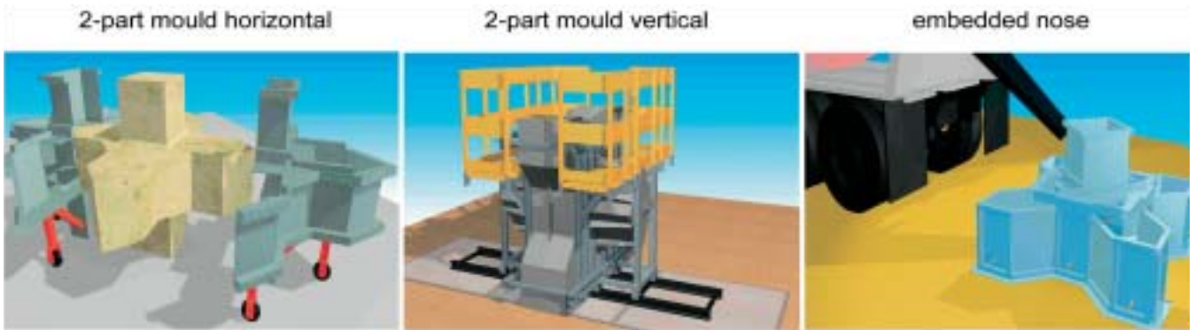
Figure 13. Various mould options for casting.
