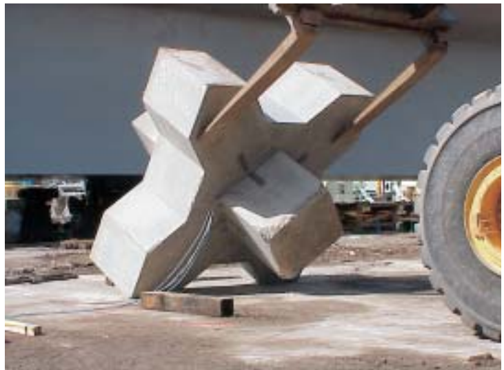
Figure 11. Tip Drop Test in reality.
